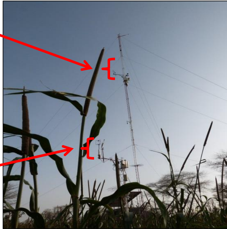
Eddy-covariance antenna (4m) + EC at 4.5m + Campbell weather station
